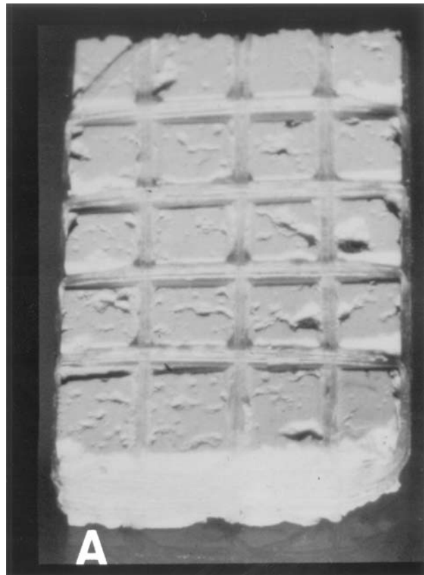
Figure 1 Reinforced porous hydroxyapatite implant sized 2 \times 3 \times 8 mm used in the study. Reinforcing poly-l/dl-lactide threads were placed in the grooves on sides facing toward the vertebral end-plates making intimate contact of hydroxyapatite and host bone possible.
